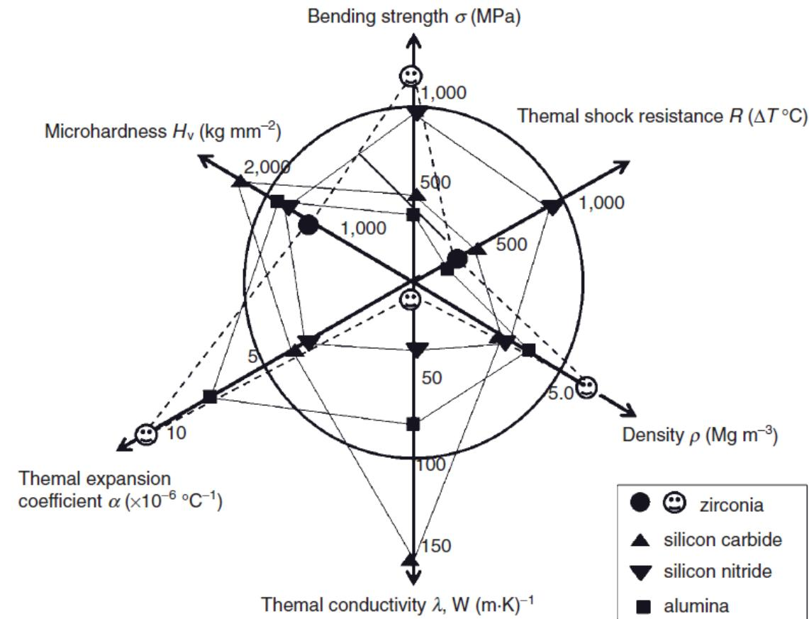
Performance-application diagram of four typical advanced structural ceramics: zirconia; silicon carbide; silicon nitride; and alumina. Owing to the dependency of the properties on processing
